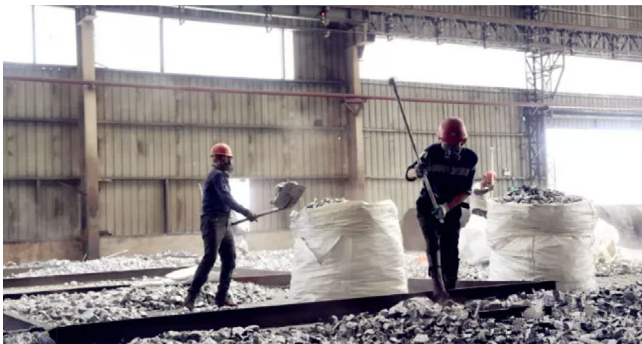
Workers manually crush silicon in Jingang Circular Economy Industrial Park, Ili Prefecture, Xinjiang. Source: Kokodala News via Weixin.
